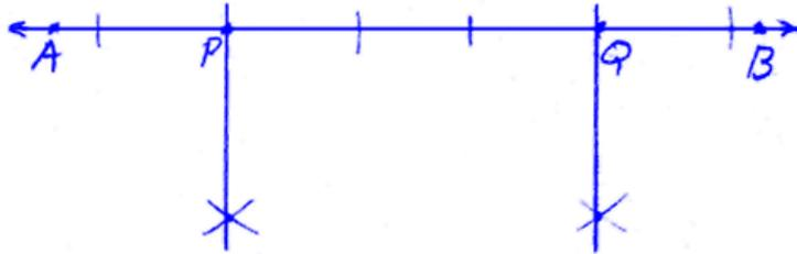
With the point of the compass at  $P$  set some convenient span on the compass, and then on the perpendicular through  $P$ , strike an arc at  $C$ .
