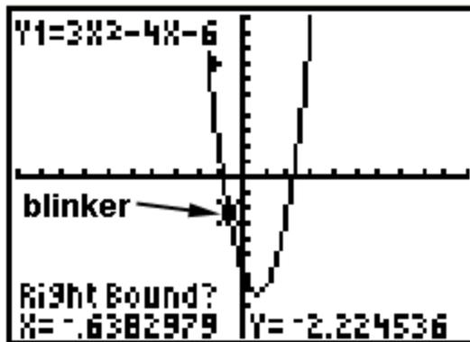
At this point another question will appear asking for the "Right Bound?". Move the blinker with the **LEFT/RIGHT ARROWS** until it is clearly to the right of the desired root. Press **ENTER**.
