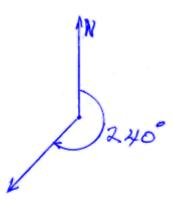
Surveying, bearing angle (the acute angle at which the direction varies to the east or west from the north-south line):
